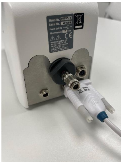
Figure 9 P-Pump Communication Cable Connection
