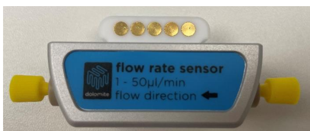
Figure 13 Example of a Flow Rate Sensor
