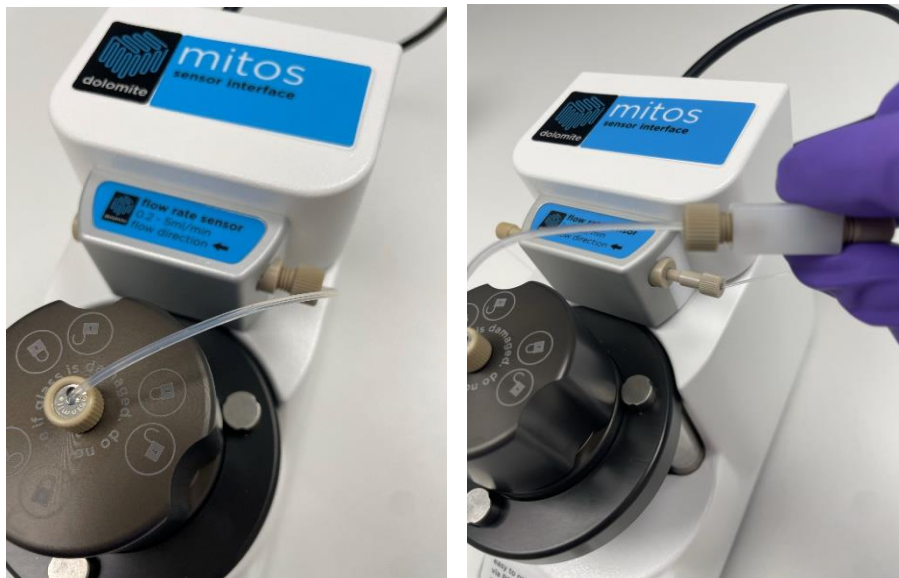
Figure 20 Fluidic Connection between P-Pump and Flow Rate Sensor when using Large Sensor (left) and Small Sensor (right)
