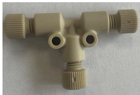
Figure 16 2-Way in-line valves and T-connectors are pre-assembled in Calibrated Tubing Network
