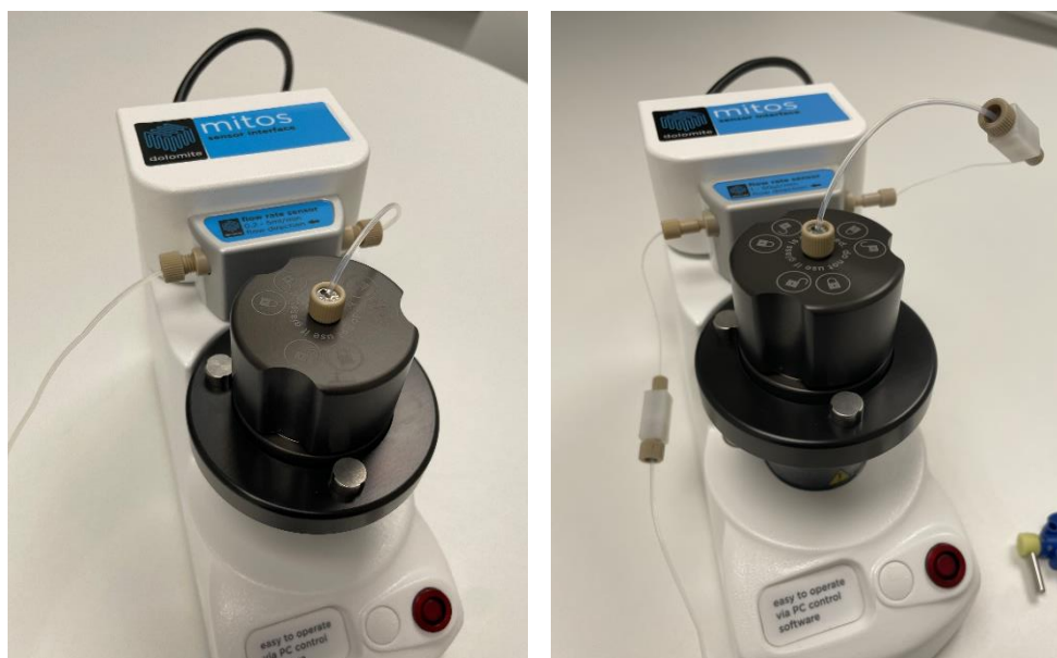
Figure 21 Fluidic Connection between Flow Rate Sensor and Linear Connector when using Large Sensor (left) and Small Sensor (right)
