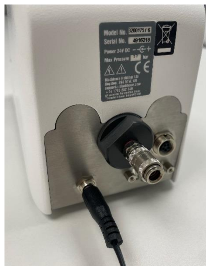
Figure 8 P-Pump Power Connection
