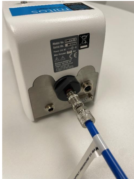
Figure 7 P-Pump pneumatic tubing connection
