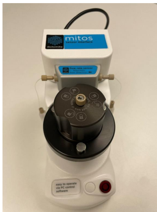
Figure 18 a) Flow Rate Sensor Convertor b) 2 Convertors connected to a Flow Rate Sensor
