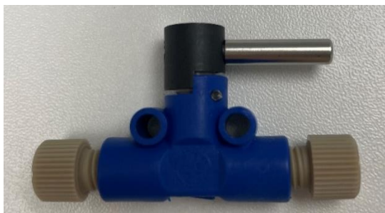
Figure 16 2-Way in-line valves and T-connectors are pre-assembled in Calibrated Tubing Network
